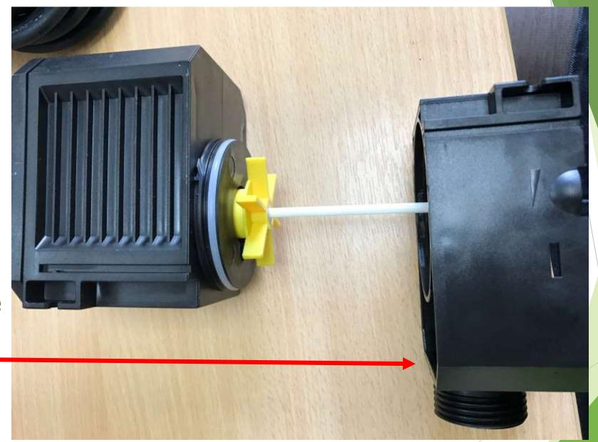
Remove the plastic casing and white pole.
