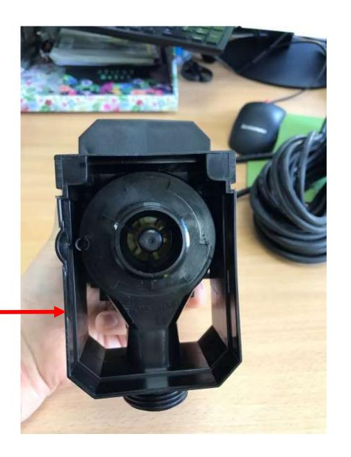
You will then be able to pull the plastic casing forwards and access to the impeller will now be possible.
